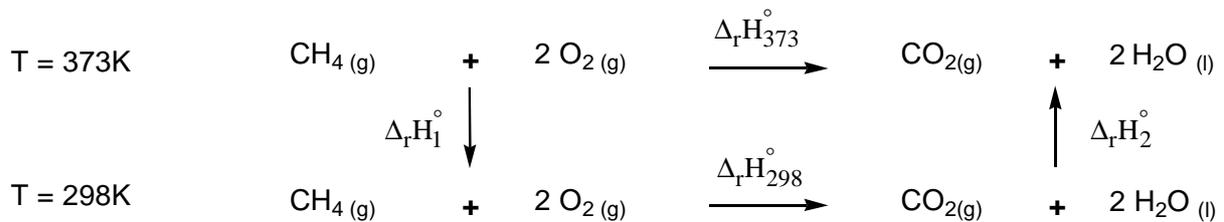
$$\text{d'où } \Delta_r H_{373}^\circ = \Delta_r H_{298}^\circ + \int_{298}^{373} \sum_i \nu_i \cdot c_{p_i} dT = -883,3 \text{ kJ} \cdot \text{mol}^{-1}$$
