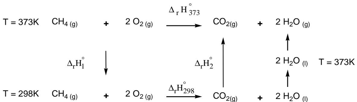
$$\text{avec } \Delta_r H_2^\circ = \int_{298}^{373} [c_p(\text{CO}_2) + 2 \cdot c_p(\text{H}_2\text{O})] \cdot dT + 2 \cdot \Delta_{\text{vap}} H^\circ(\text{H}_2\text{O})$$
